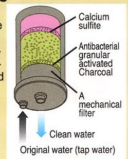
Filter change will be notified by the LCD. voice or alarm sound (Jr. II does not)lead, chloline, rust, muddiness, and does not eliminate important mineral. Filter change will be notified by the LCD. voice or alarm sound (Jr. II does not) have sound notification.
