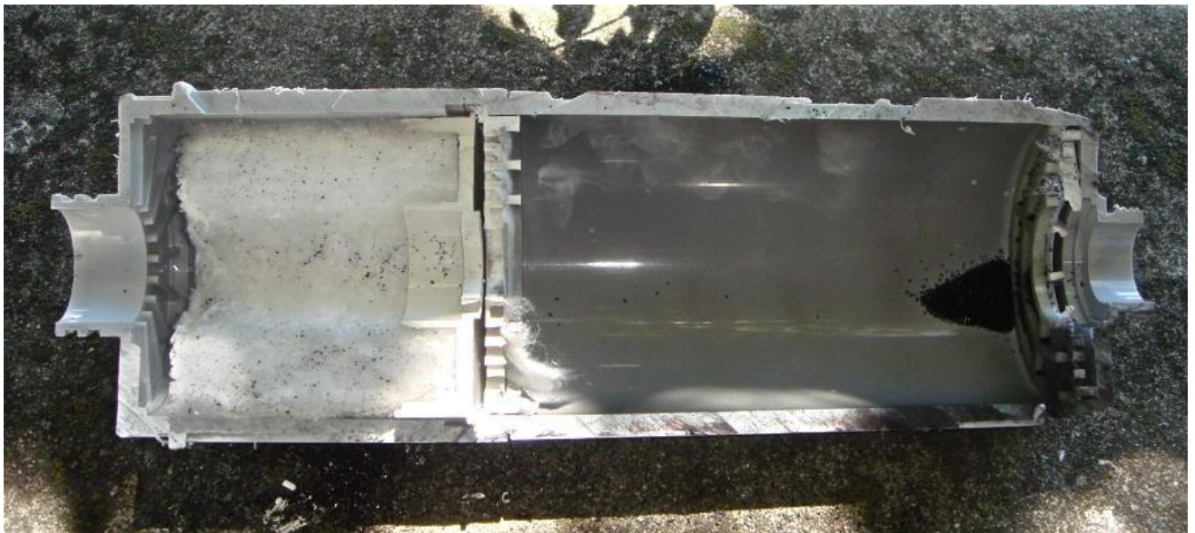
Figure 7 – LifeIonizer Filter Cross Section Cut – Resting on its Granulated Carbon
